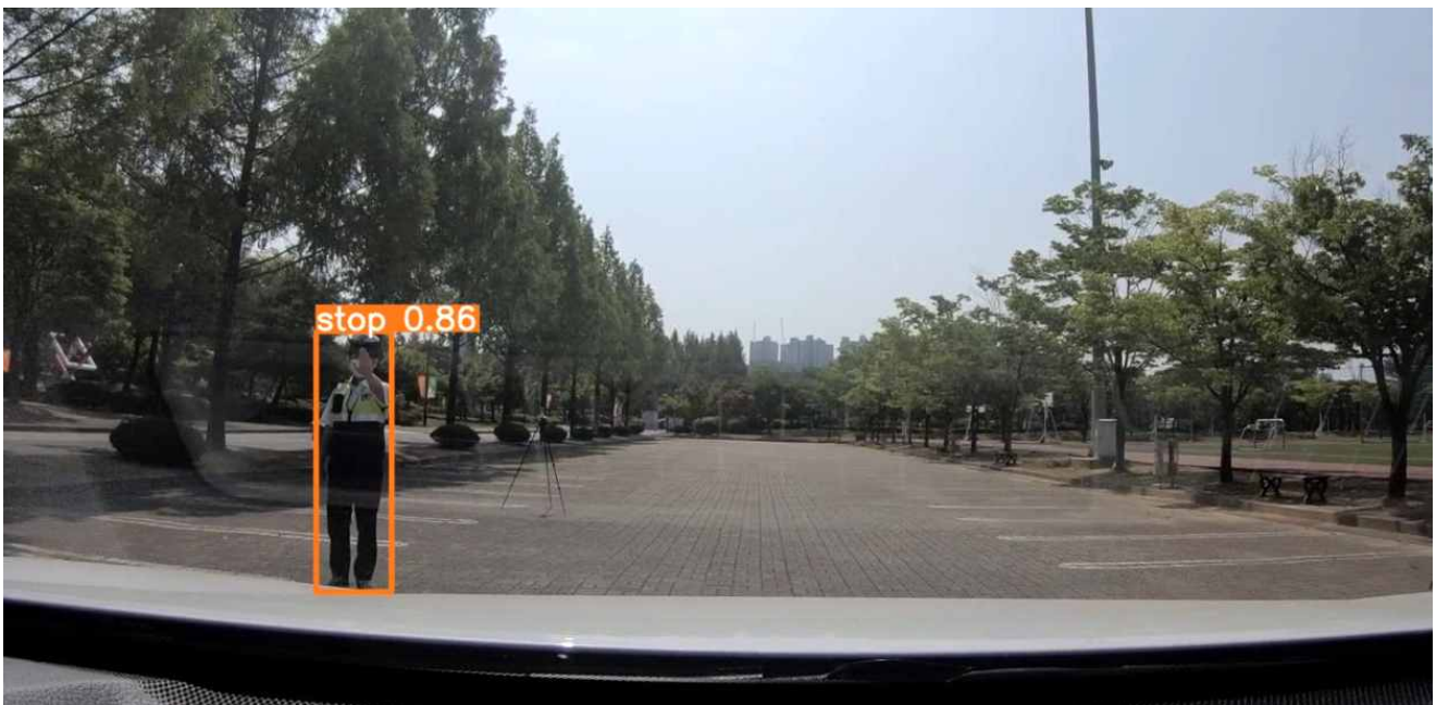
▲ Vehicle recognition of hand signal for traffic stop (front): Recognition of hand signal stop through vehicle camera equipped with hand signal recognition AI technology developed by the research team
