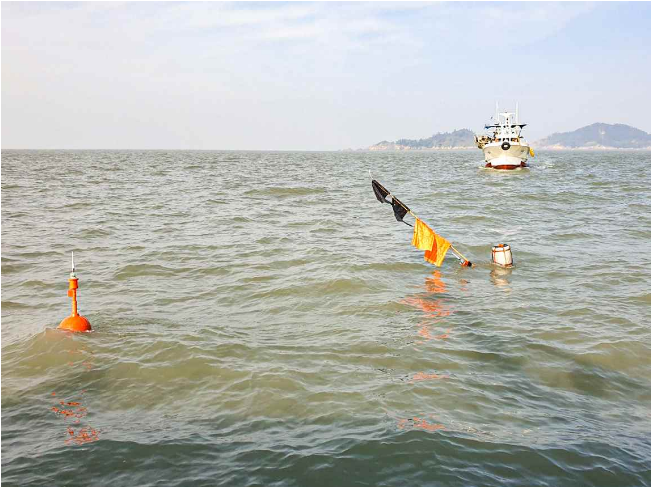
▲ Attachment of fishing gear automatic identification buoy and operation of demonstration test: Conduct a demonstration test of fishing gear management by attaching an electronic buoy for automatic identification of fishing gear to the coastal gill net
