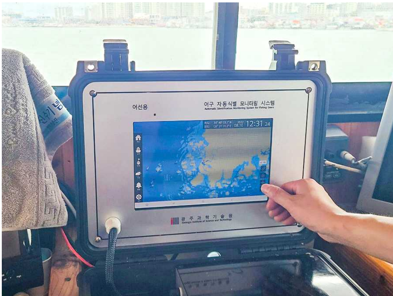
▲ Demonstration test operation of automatic identification monitoring system for fishing gear: Monitoring by installing a control system on fishing vessels
