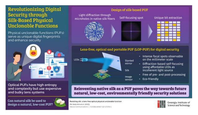
The first natural physical unclonable function (PUF) for environmentally friendly digital security The new PUF takes advantage of the diffraction of light through natural microholes in native silk to create a secure and unique digital key for future security solutions
