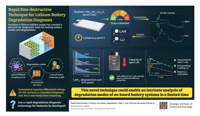
Lithium-ion batteries lie at the heart of all modern electronics and are now being increasingly implemented in electric vehicles. As a result, there has been a rapid increase in its usage, and, with it, a growing demand for tools to test the "state of health" (SOH) of these batteries reliably. This is particularly important in light of the fact that understanding degradation symptoms in batteries is vital for improved maintenance and accident prevention due to malfunctions.
